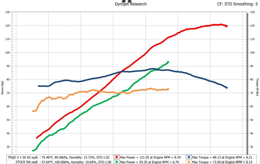
Engine RPM (rpmx1000)
